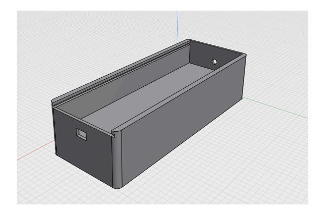
There are two cutouts in the housing design. The rectangular hole is for the on/off switch, allowing users to easily enable or disable the alarm system. The circular hole is positioned to align with the mini piezo buzzer, allowing the sound to pass clearly through the enclosure for effective audio alerts.
