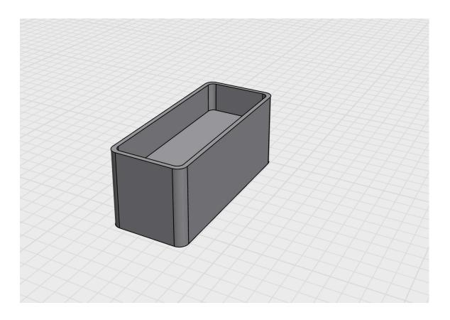
This is the magnet holder, designed to be mounted on the door frame, positioned close to the main housing. The main housing, which contains the electronics, is mounted on the moving part of the door. When the door is closed, the magnet aligns with the reed switch in the main housing to maintain the circuit's inactive state. Opening the door causes the magnet to move away, triggering the alarm.
