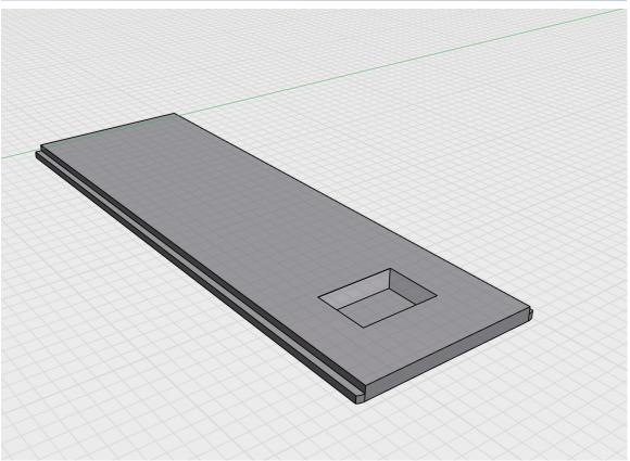
This is the sliding lid for the main housing. We designed a chambered cutout to provide users with a convenient grip area, making it easy to slide the lid open or closed. Additionally, the rails were precisely cut and fitted to ensure the lid aligns securely with the housing, forming a tight seal that helps prevent water and dirt from entering and damaging the internal components.
